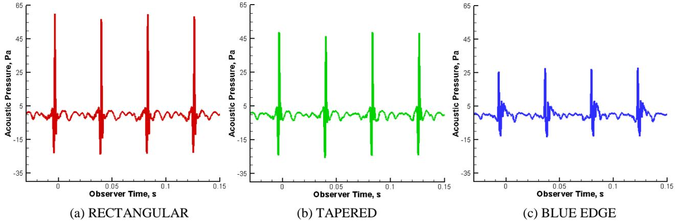
Figure 14. Acoustic pressure time history at azimuth angle  $\psi = 125$ , elevation angle  $\theta = -45^\circ$  below the rotor plane, and radius of 30.48m from the helicopter c.g. (i.e.. the location of the black dot in Figure 13).
