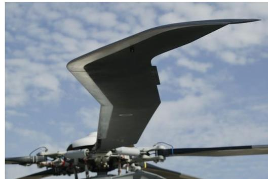
Figure 9. Blue Edge blade concept from Eurocopter (now Airbus Helicopters).<sup>16</sup>
