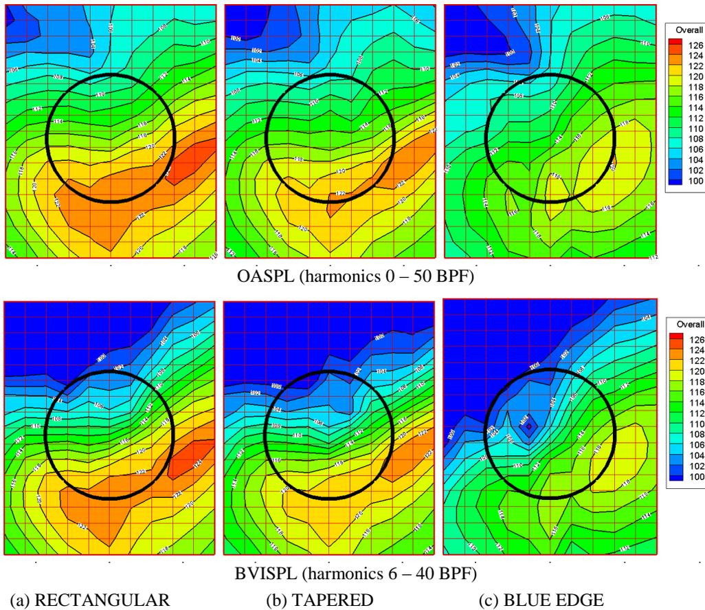
Figure 11. CHARM/PSU-WOPWOP main rotor OASPL and BVISPL predictions one rotor radius beneath the nominal Bell 430 rotor for the three blade geometries;  $\alpha_s=6^\circ$  (back),  $\mu=0.15$  and  $C_T=.00143$ . The black circle represents the rotor tip – advancing side on the right.
