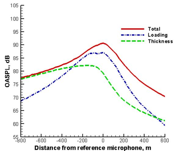
Figure 7. Noise components and their contribution to the OASPL predictions for a 100 kts flight case flown at 150 m altitude.
