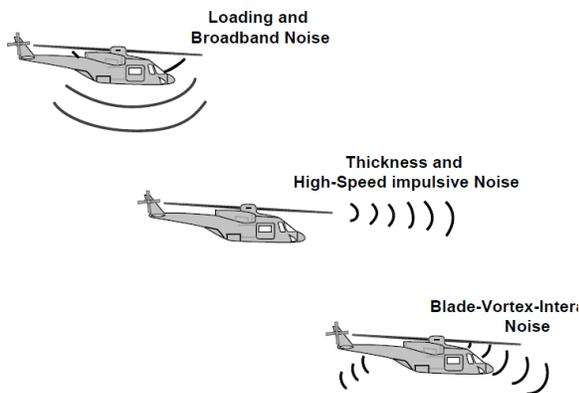
Figure 6. Typical direction of primary radiation for various rotor noise sources.
