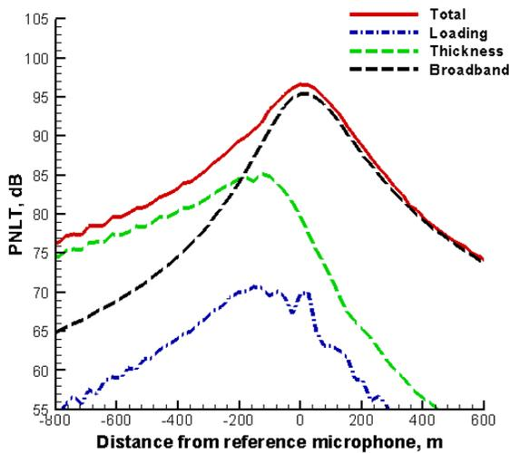
Figure 8. Noise components and their contribution to the PNL T predictions for a 100 kts flight case flown at 150 m altitude.
