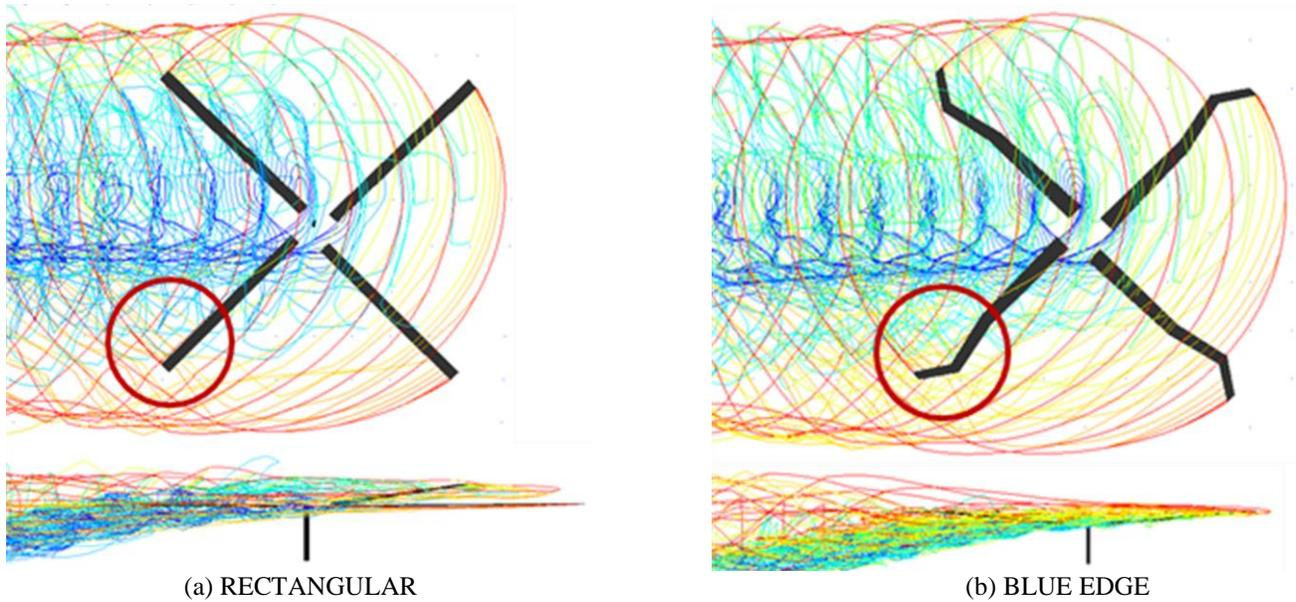
Figure 12. BVI event as predicted by CHARM for the baseline RECTANGULAR blade and the BLUE EDGE blade.
