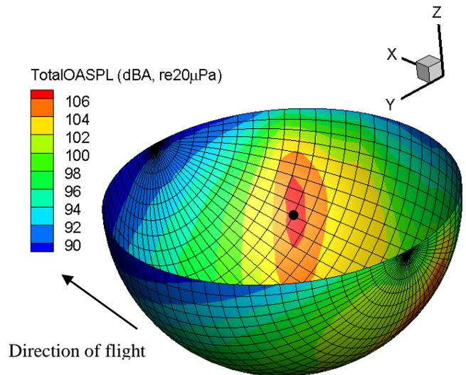
Figure 13. Contours of OASPL on a 30.48m radius hemisphere, centered at the Bell 430 c.g. location. The hemisphere follows the aircraft. OASPL contours shown are for the standard rectangular blades.
