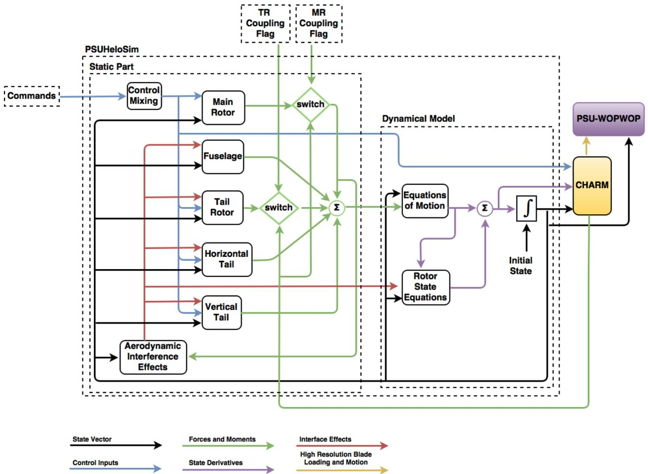
Figure 1. Schematic of the PSUHeloSim/CHARM/PSU-WOPWOP simulation model.
