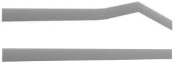
Figure 6.2. Tapered and Blue Edge-like planforms.
