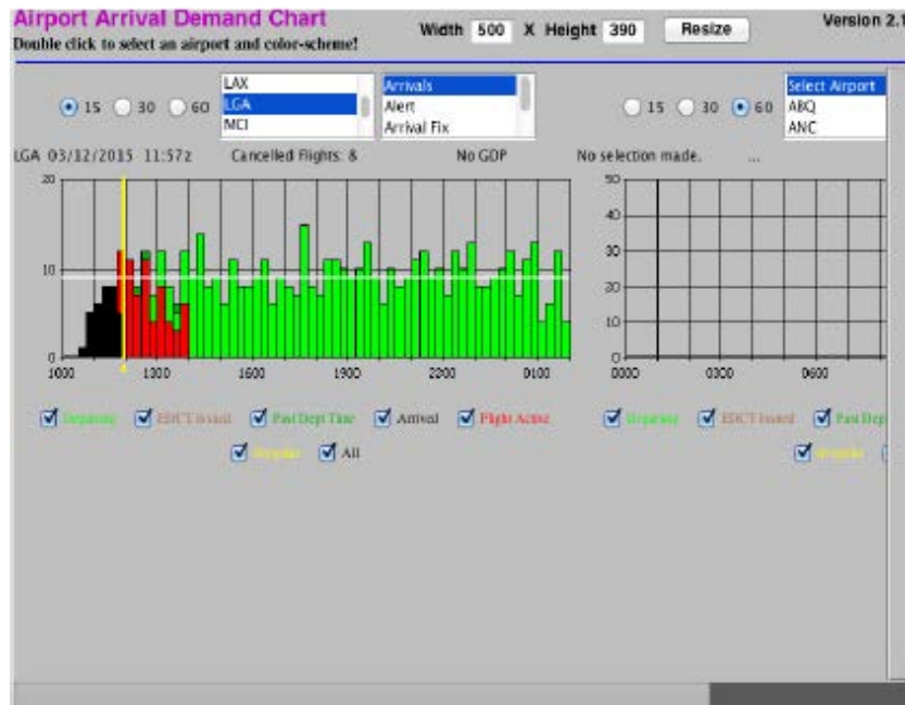
Figure 5. Airport Arrival Demand Chart for LGA on 3/12/2015. The bars indicate how many aircraft will be approaching LGA for landing during each 15-minute time window.
