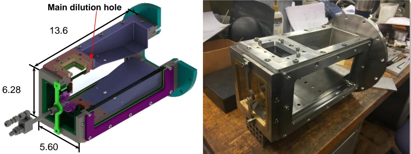
**Figure 6. High altitude relight combustor model (left) and completed rig (right).** *The high altitude relight combustor replicates the key geometry and flow features of the referee rig, including dilution jet hole placement, overall size, swirler geometry, and injector geometry.*
