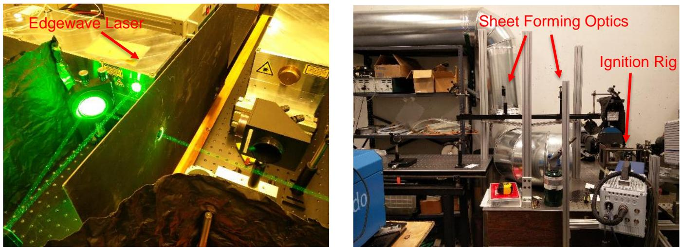
**Figure 5.** Edgewave pump laser (left) and dye laser with sheet forming optics, and the ignition rig
