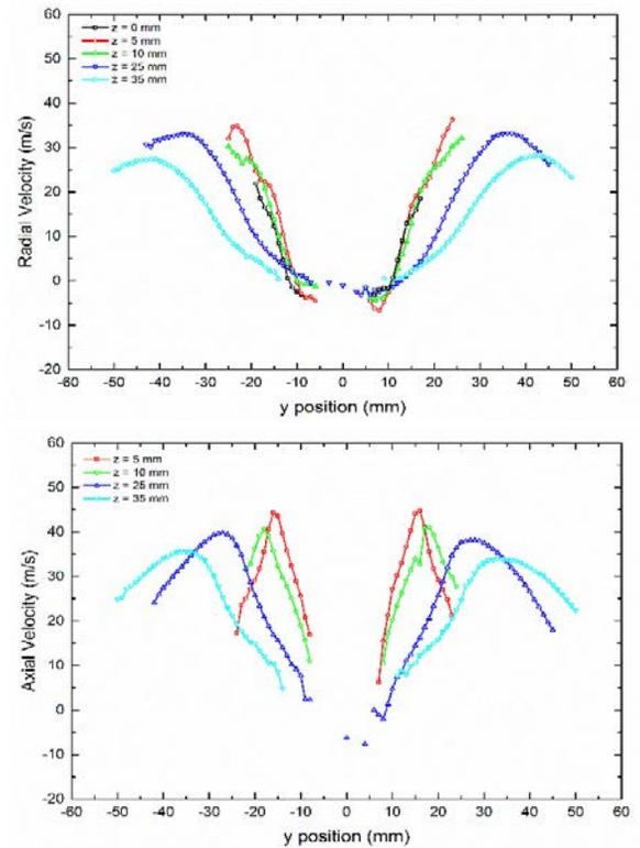
**Figure 17. A-2 fuel droplet mean radial and axial velocity. Mean radial velocity plotted against  $y$  position (top) and mean axial velocity plotted against  $y$  position (bottom) at various distances from the deflector plate**
