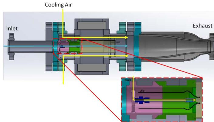
Figure 5. High shear swirl combustor, showing a) pressure vessel instrumented for high speed stereo PIV and OH PLIF, and b) a cross section with generic swirler holder/injector for illustrative purposes
