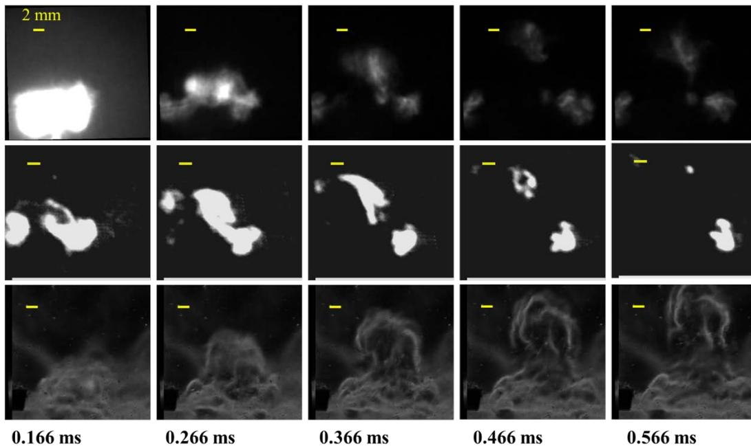
Figure 7. Top row) emission imaging, middle row) OH PLIF imaging, bottom row) Schlieren imaging of an evolving ignition kernel.
