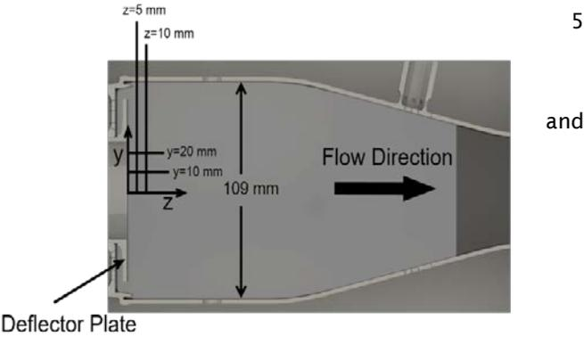
**Figure 15. Cutaway of the single cup referee combustor. The origin is taken to be at the intersection of centerline of the combustor with the front plane of the deflector plate as marked.**
