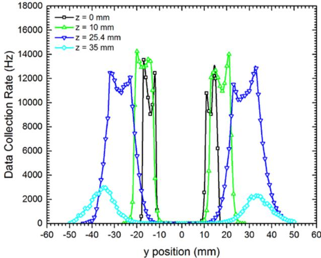
**Figure 14. A-2 data collection rate. Data collection rate versus y-position at various axial locations for A-2 at  $\phi=0.096$**
