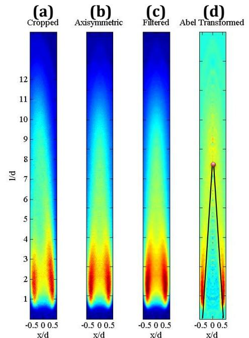
**Figure 9. Step-by-step summary of image processing approach:(a) time-averaged, background subtracted and cropped (b) Axisymmetric (c) 2-D median filtered (d) Abel transform with  $\langle c \rangle = 0.5$  contour drawn.**
