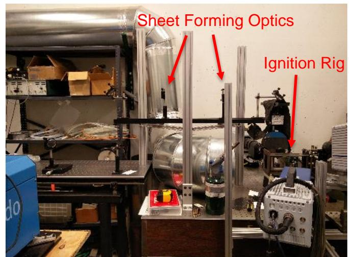
Figure 19. Edgewave pump laser (left) and dye laser with sheet forming optics, and the ignition rig
