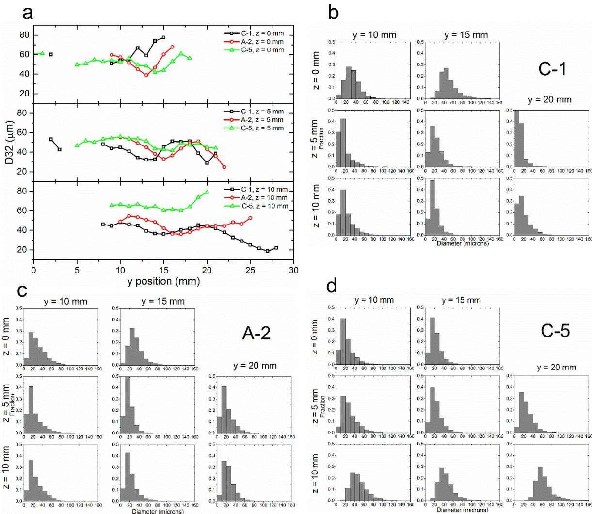
**Figure 16. Sauter mean diameter and representative diameter histograms a) Sauter mean diameter plotted versus  $y$  position for each fuel 0 mm, 5 mm, and 10 mm downstream of the deflector plate for comparison b) C1 diameter histograms, c) A2 diameter histograms and d) C5 diameter histograms at  $y = 10$  mm, 15mm, and 20 mm**
