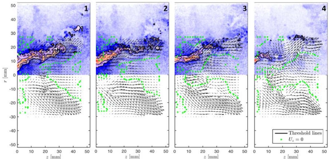
Figure 4. Film-strip of processed detailed diagnostic data, showing OH-PLIF (blue), fuel-PLIF (red), mixture of fuel and OH (purple), and in-plane velocity field (black). Green line indicates contour of zero in/out of plane velocity.
