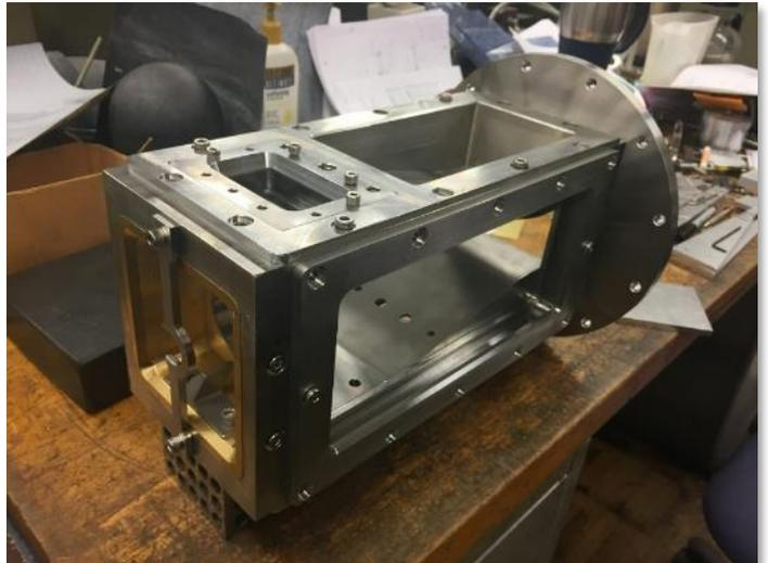
**Figure 20. High altitude relight combustor model (left) and completed rig (right). The high altitude relight combustor replicates the key geometry and flow features of the referee rig, including dilution jet hole placement, overall size, swirler geometry, and injector geometry.**
