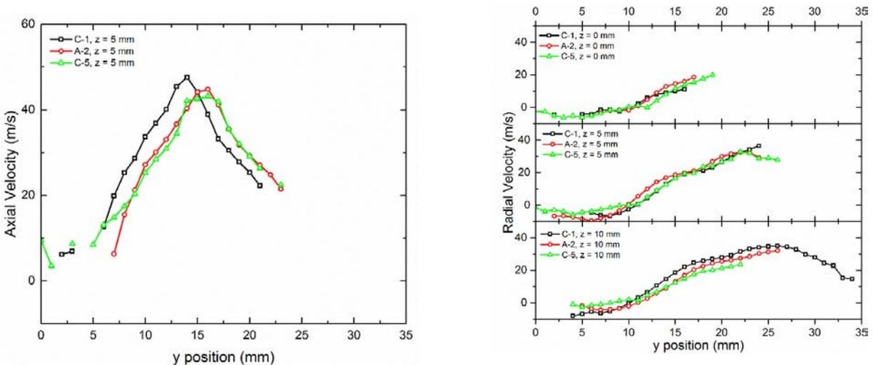
**Figure 18. Axial and radial velocity profiles. a) Axial velocity plotted versus  $y$  position for each fuel 5 mm downstream of the deflector plate and b) radial velocity plotted as a function of  $y$  position at 0 mm, 5 mm, and 10 mm downstream of the deflector plate for each fuel**
