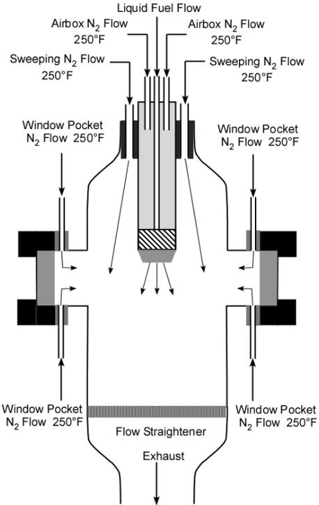
Figure 2. Schematic diagram of the RTS test rig.
