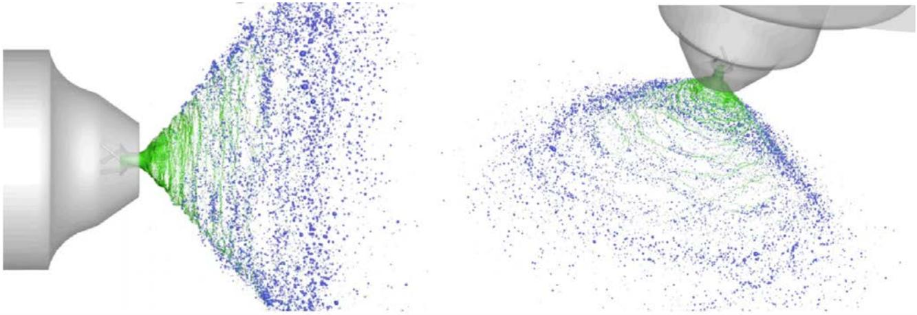
Figure 11: Representative simulation results. The iso-surface of VoF variable = 0.5 is shown in green and the Lagrangian particles is shown as blue spheres whose size is scaled based on the droplet diameter.
