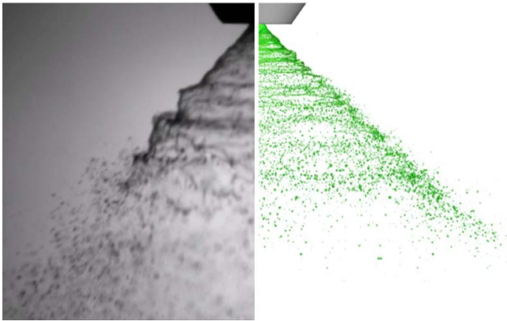
Figure 12: Comparison between numerical simulation and experiment. The image on the left was taken by high-speed camera in the experiment. Simulation results of iso-surface = 0.5 and Lagrangian particles scaled by droplet size are both colored in green shown on the right.
