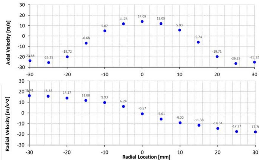
Figure 5. Axial and radial velocities for fuel A2 as a function of radial position. Note the central recirculation zone from -12 mm to +12 mm positive axial velocities (towards the nozzle).
