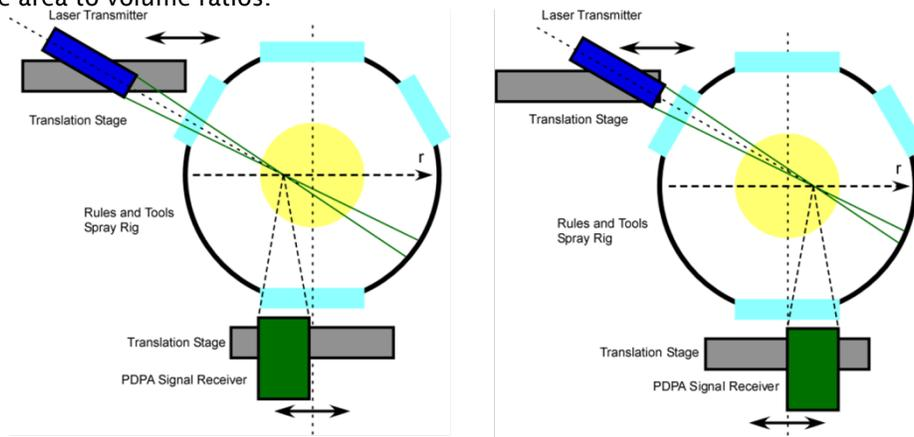
Figure 3. Top view of PDPA measurement geometry.
