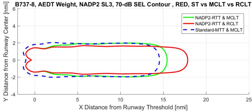
**Figure 56:** B737-800 Noise Contour Comparison at SEL 70dB for Stage Length 3 NADP2
