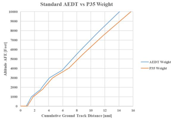
Figure 16: STANDARD AEDT vs. Project 35 Weight for Stage Length 3
