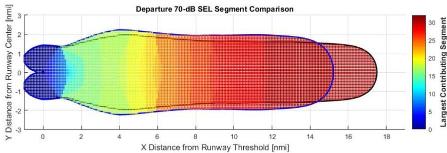
**Figure 52:** Detailed B737-800 Noise Contour Comparison at SEL 70dB at Stage Length 3 NADP-1
