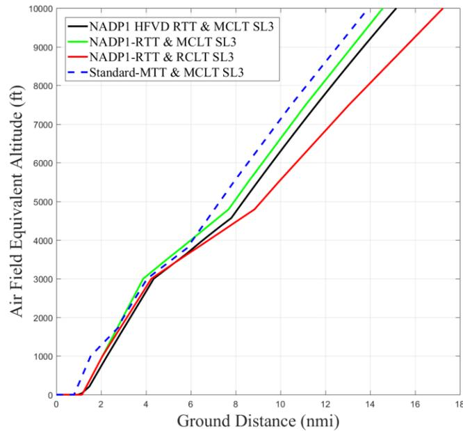
**Figure 47:** Altitude vs Ground Distance for B737-800 Trajectory Comparison for Stage Length 3 NADP1
