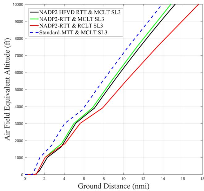
Figure 55: Altitude vs Ground Distance for B737-800 Trajectory Comparison for Stage Length 3 NADP2
