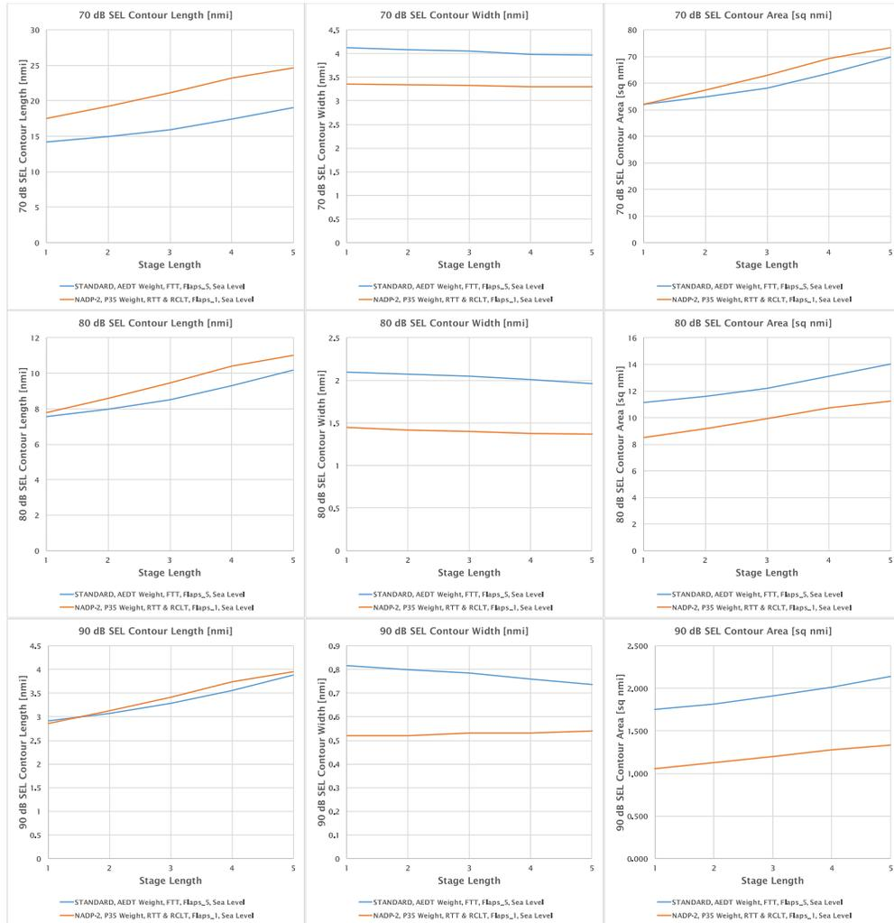
Figure 40: Procedure, Weight and Thrust Sensitivity Noise Results
