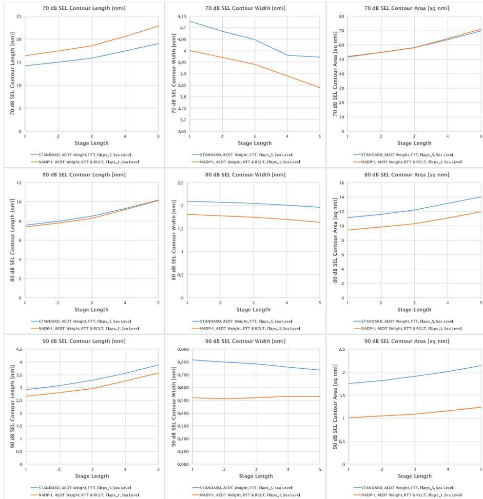
Figure 34: Procedure and Thrust Sensitivity Noise Results
