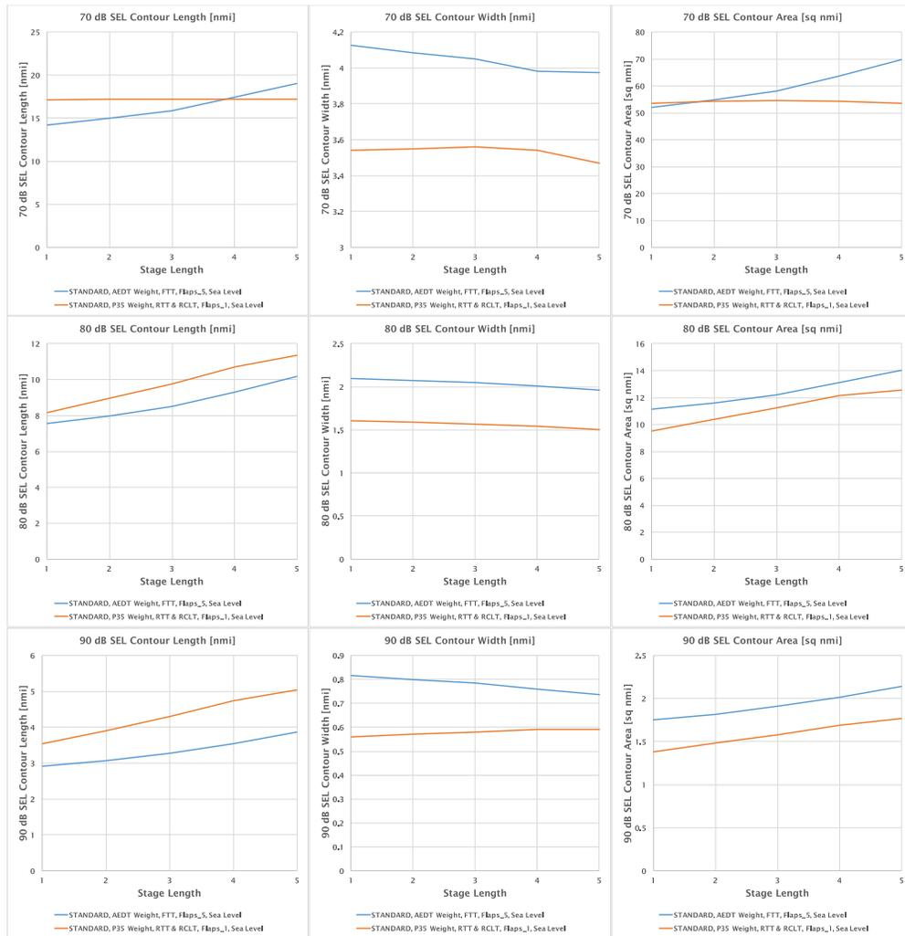
**Figure 22: Weight and Thrust Sensitivity Noise Results**
