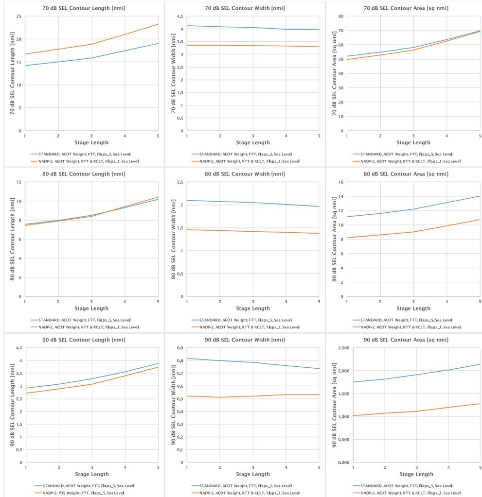
Figure 36: Procedure and Thrust Sensitivity Noise Results
