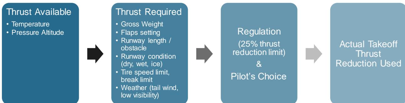
**Figure 42. Four Factors of Takeoff Thrust Determination**
