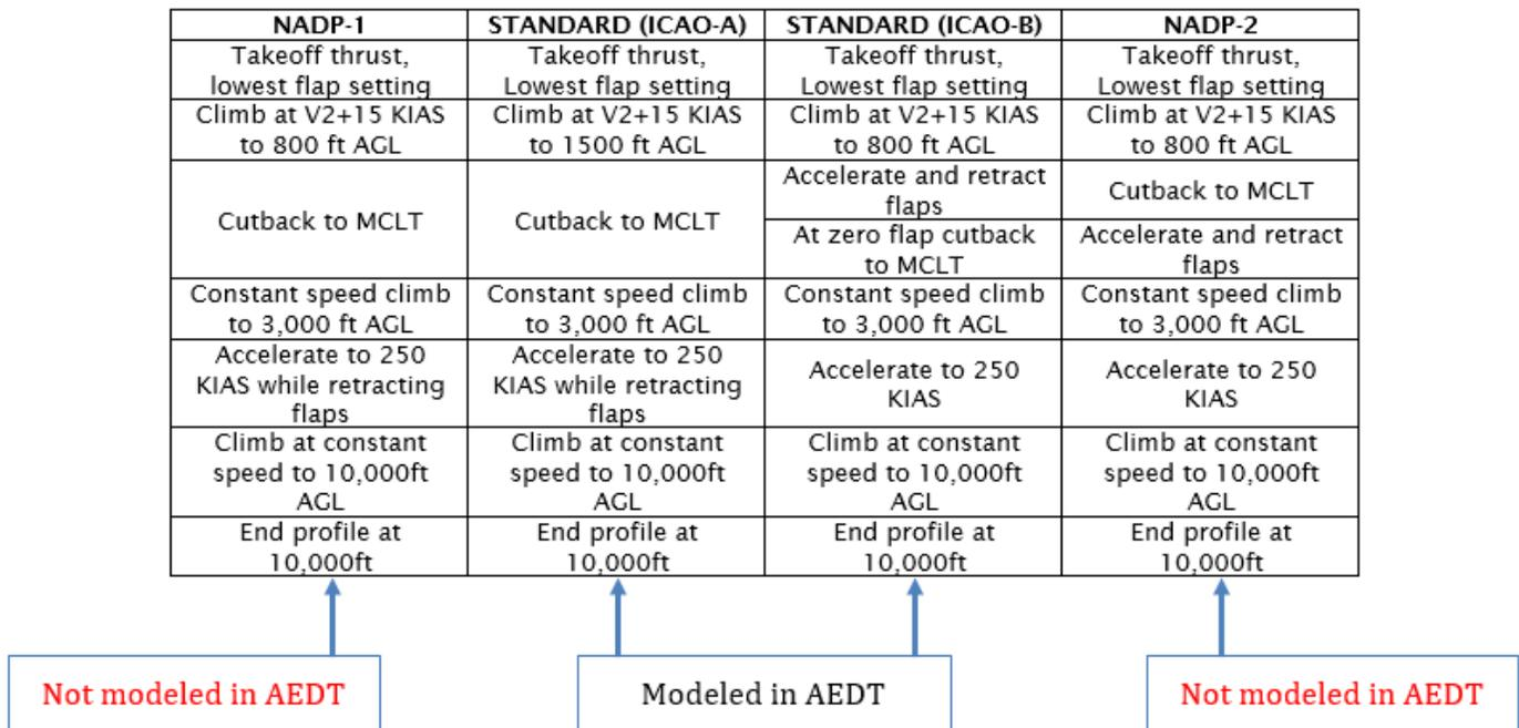
**Figure 23: STANDARD and NADPs Procedures**
