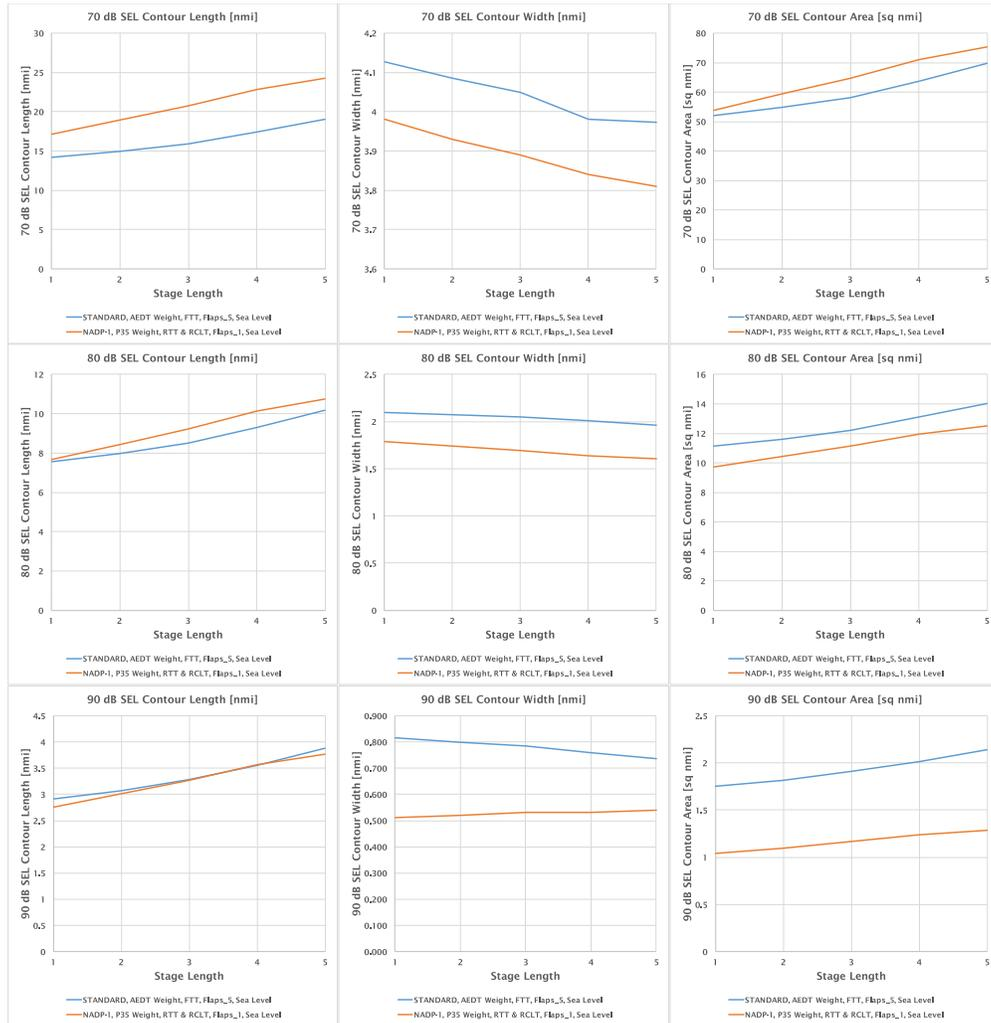
Figure 38: Procedure, Weight and Thrust Sensitivity Noise Results
