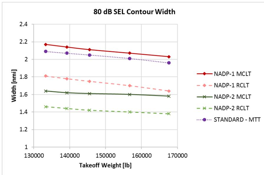
Figure 64: B737-800 Contour Width Comparison for SEL 80dB
