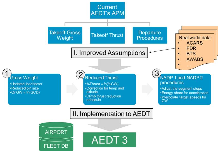
**Figure 41.** A Two-Step Approach to Improve AEDT's Modeling Accuracy
