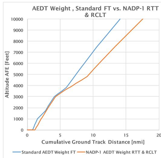
Figure 33: AEDT Weight, STANDARD FT vs NADP-1 RTT & RCLT
