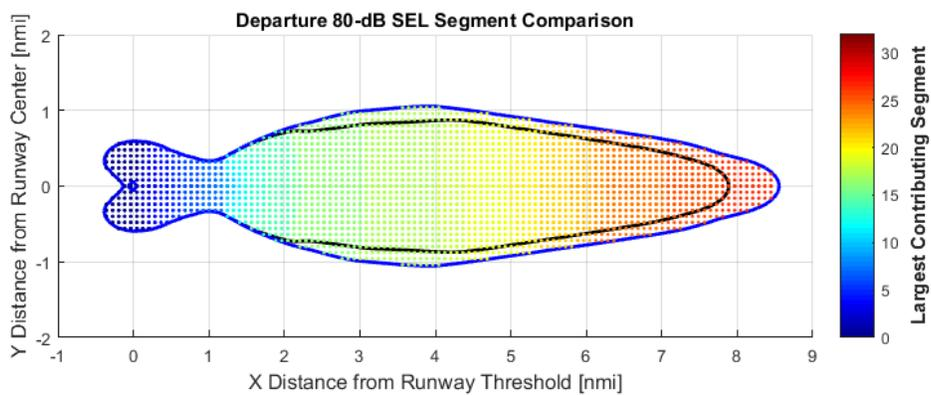
**Figure 53:** Detailed B737-800 Noise Contour Comparison at SEL 80dB at Stage Length 3 NADP-1
