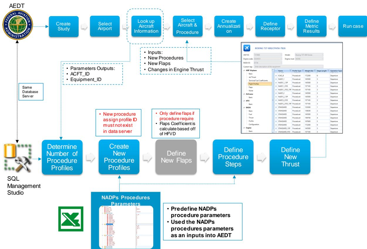
Figure 46. Process of Adding NEW GW, Thrust, and Procedures to AEDT
