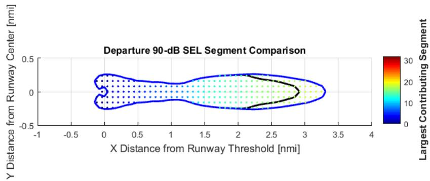
**Figure 62:** Detailed B737-800 Noise Contour Comparison at SEL 90dB at Stage Length 3 NADP-1
