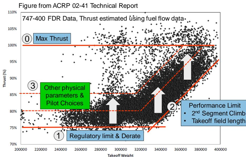
Figure 43. Schematic Diagram of the Takeoff Thrust Model
