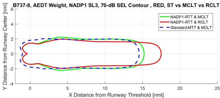
**Figure 48:** B737-800 Noise Contour Comparison at SEL 70dB for Stage Length 3 NADP1
