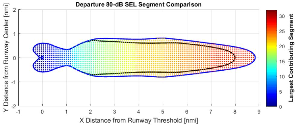
**Figure 61:** Detailed B737-800 Noise Contour Comparison at SEL 80dB at Stage Length 3 NADP-2
