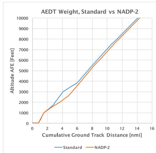
**Figure 27: AEDT Weight STANDARD vs NADP-2 Procedure for Full Thrust**
