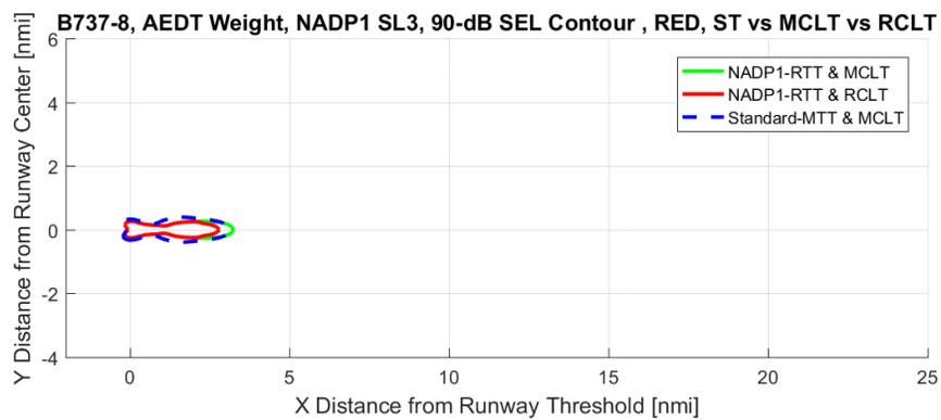
**Figure 50:** B737-800 Noise Contour Comparison at SEL 90dB for Stage Length 3 NADP1
