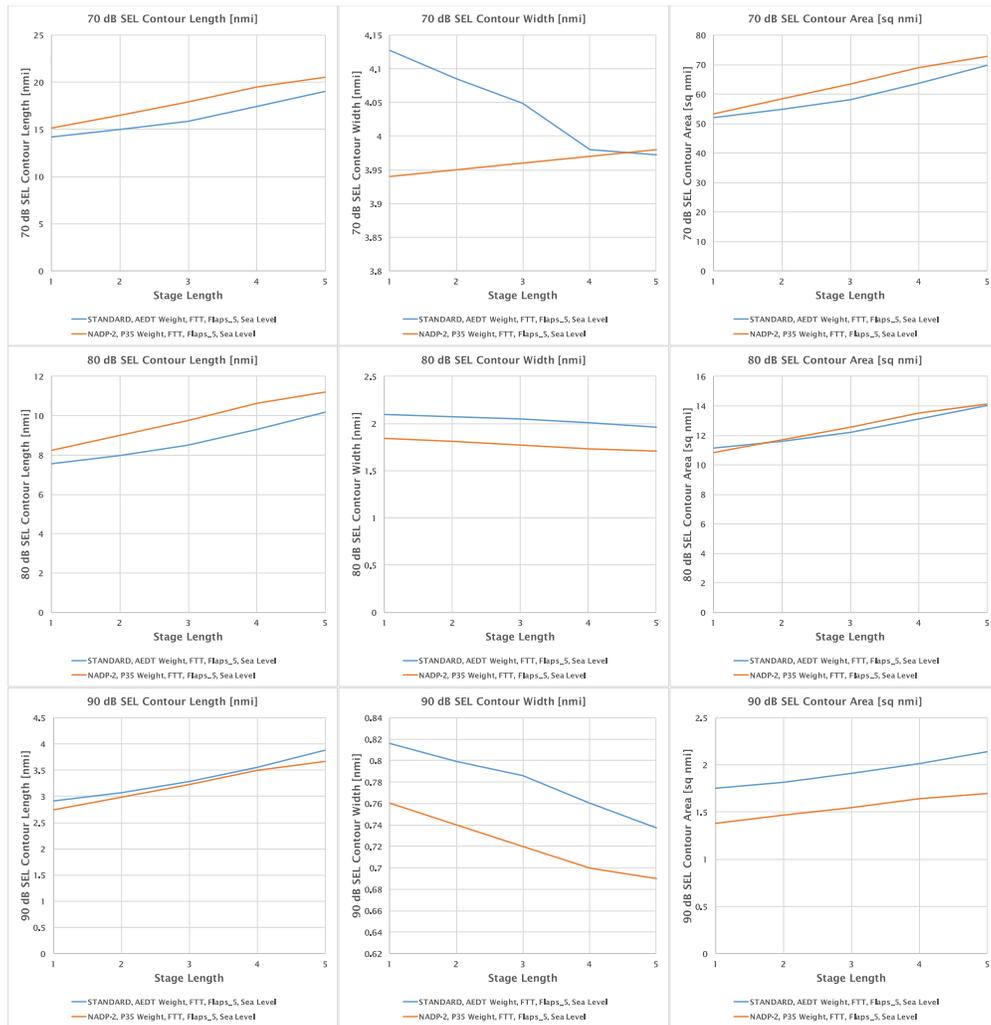
Figure 32: Procedure and Weight Sensitivity Noise Results
