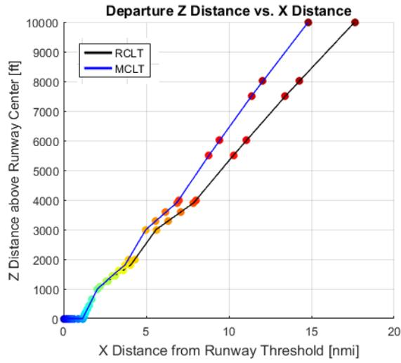
**Figure 59:** Detailed Altitude vs Ground Distance for B737-800 Stage Length 3 NADP-2
