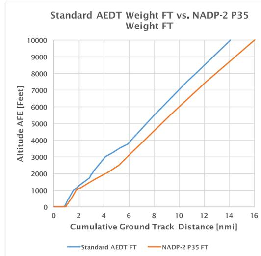
Figure 31: STANDARD AEDT Weight FT vs NADP-2 P35 Weight for Full Thrust
