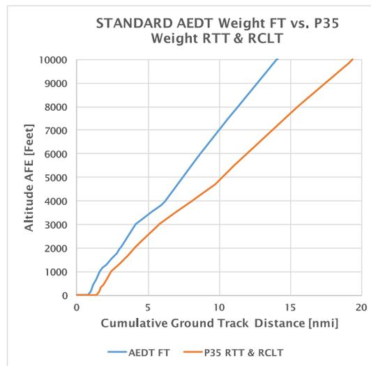
**Figure 21:** STANDARD AEDT Weight FT vs. Project 35 Weight RTT & RCLT for Stage Length 3
