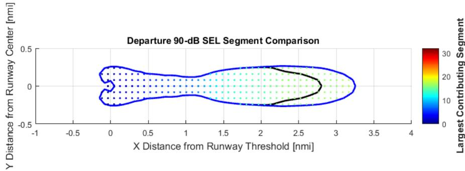
Figure 54: Detailed B737-800 Noise Contour Comparison at SEL 90dB at Stage Length 3 NADP-1
