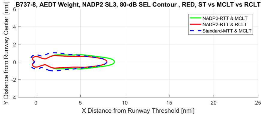
**Figure 57:** B737-800 Noise Contour Comparison at SEL 80dB for Stage Length 3 NADP2
