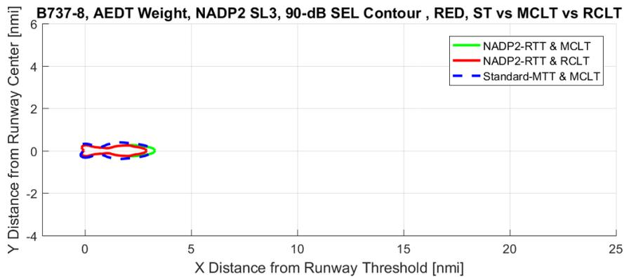
**Figure 58:** B737-800 Noise Contour Comparison at SEL 90dB for Stage Length 3 NADP2
