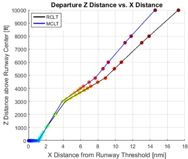
**Figure 51:** Detailed Altitude vs Ground Distance for B737-800 Stage Length 3 NADP-1
