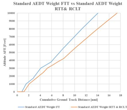
Figure 19: STANDARD Procedure for AEDT Weight Full vs Reduced Takeoff Thrust Trajectory for Stage Length 3
