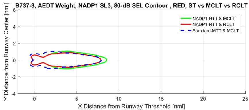
**Figure 49:** B737-800 Noise Contour Comparison at SEL 80dB for Stage Length 3 NADP1
