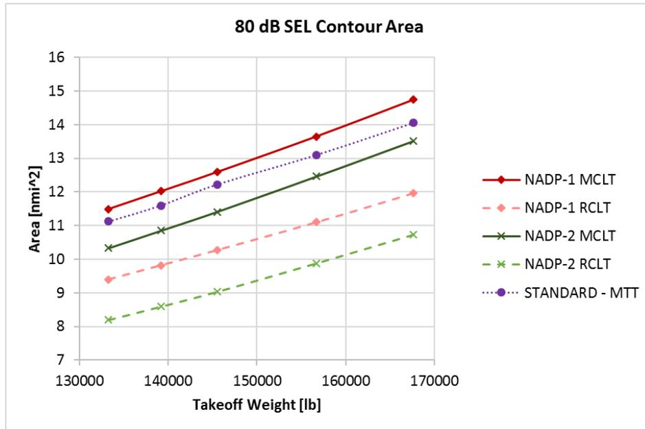
Figure 65: B737-800 Contour Area Comparison for SEL 80dB
