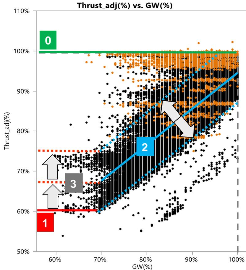
Figure 45. %Thrust<sub>adj</sub> vs %GW for B737-800
