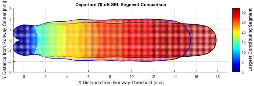
**Figure 60:** Detailed B737-800 Noise Contour Comparison at SEL 70dB at Stage Length 3 NADP-2
