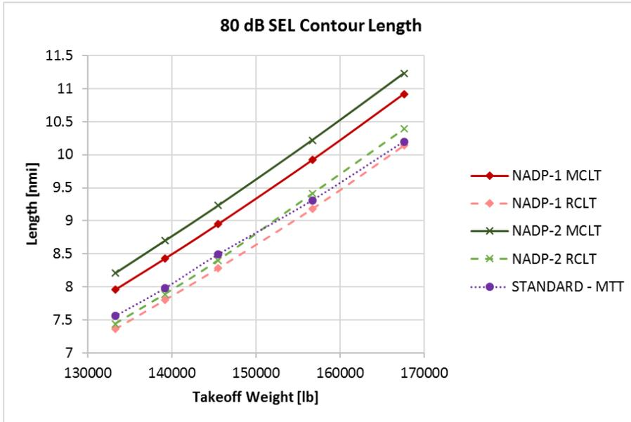
Figure 63: B737-800 Contour Length Comparison for SEL 80dB
