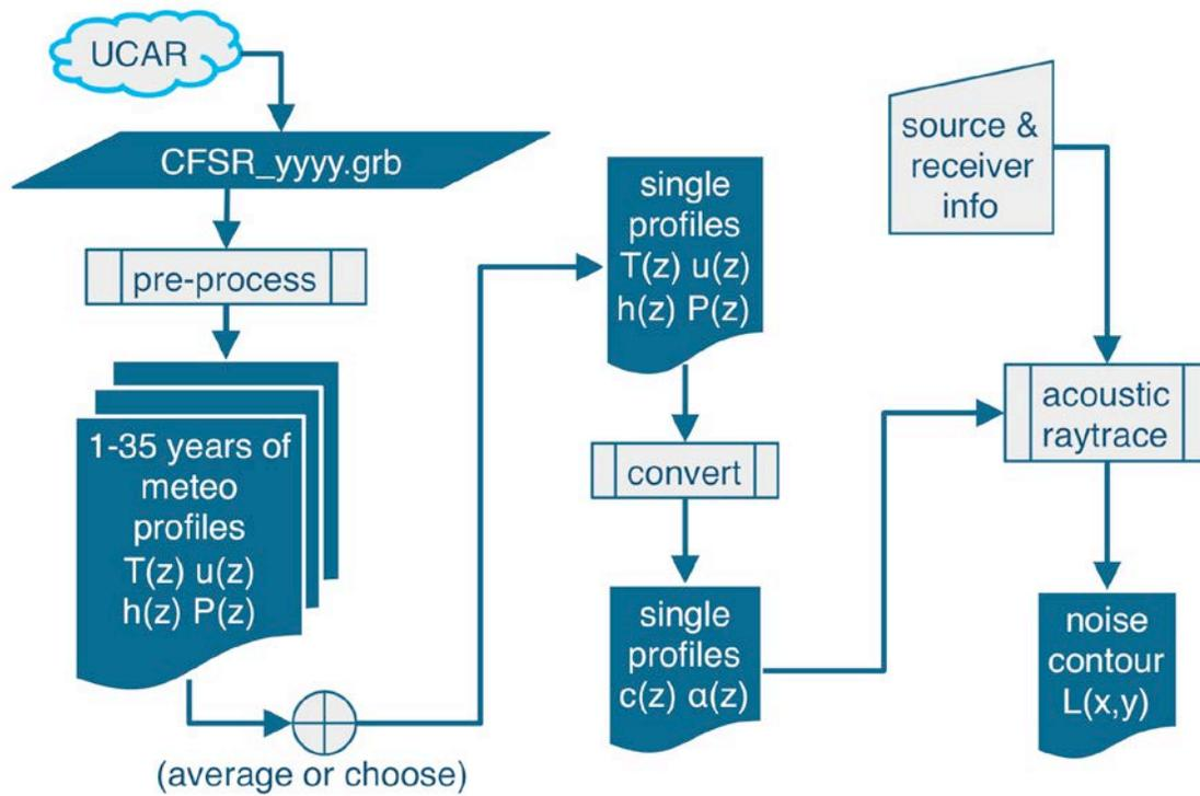
Fig. 5.4: Proposed method for integrating CFSR atmospheric data into a noise model. The meteorological profile parameters are temperature (T), wind speed and direction (u), humidity (h), ambient pressure (P). The profiles required by the acoustic ray tracing program are sound speed (c) and acoustic absorption coefficient ( $\alpha$ ). The independent variable for each profile is altitude (z).
