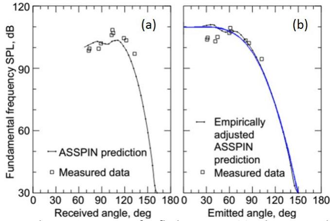
Fig. 5.5: NASA PTA aircraft source directivity pattern for flight series 100. The received angle is transformed into the emitted angle for usage in the emission time coordinate ray model. The blue curve is the approximated directivity pattern used in our analysis.
