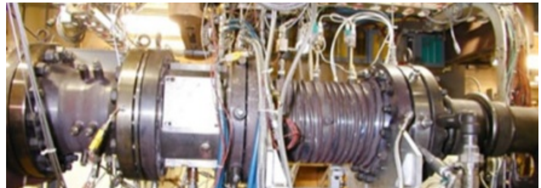
NASA Test Cell Ce-5 Stand 1 tested N+3 combustor with JetA and alternative fuel blend
