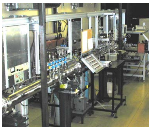
Figure 1a. Stanford 15 cm diameter shock tube. Figure 1b. Schematic of shock tube/laser absorption setup. Simultaneous measurement of multiple species time-histories and temperature with microsecond time resolution are enabled using this arrangement. Only a partial list of accessible species is indicated.
