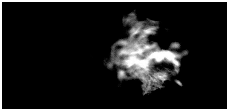
Figure 3. Sample flame chemiluminescence image from n-dodecane burning at 300 K air preheat temperature.
