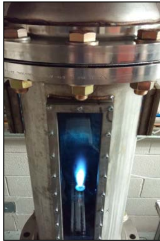
Figure 12. Picture of flame operating in pressure vessel at sub-atmospheric conditions
