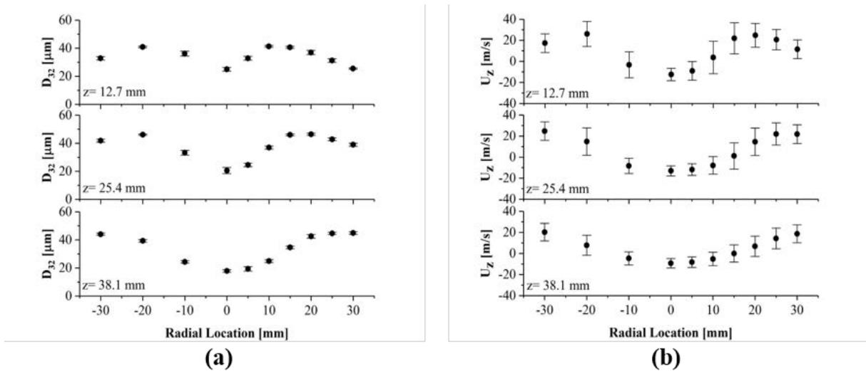
**Figure 5.** Comparisons of  $D_{32}$  and  $U_z$  distributions for C-3 at different measurement planes at  $\Delta P/P = 3\%$ ,  $T_{fuel} = 238$  K,  $T_{gas} = 238$  K at 25.4 mm measurement plane. Vertical bars on velocity represent RMS.
