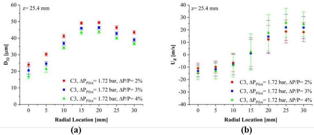
**Figure 8.** Comparisons of  $D_{32}$  and  $U_z$  distributions for C-3 when  $\Delta P/P = 2, 3, 4 \%$ ,  $T_{\text{fuel}} = 238$  K, and  $T_{\text{gas}} = 238$  K at 25.4 mm measurement plane. Vertical bars on velocity represent RMS.
