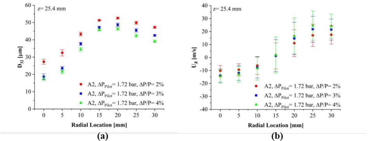
**Figure 6.** Comparisons of  $D_{32}$  and  $U_z$  distributions for A-2 when  $\Delta P/P = 2, 3, 4\%$ ,  $T_{fuel} = 238$  K, and  $T_{gas} = 238$  K at 25.4 mm measurement plane. Vertical bars on velocity represent RMS.
