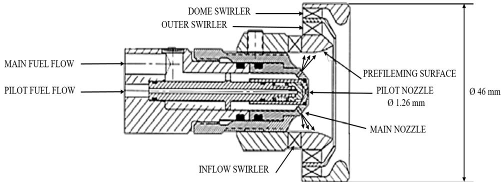
Figure 3. Schematic of the hybrid airblast pressure-swirl atomizer
