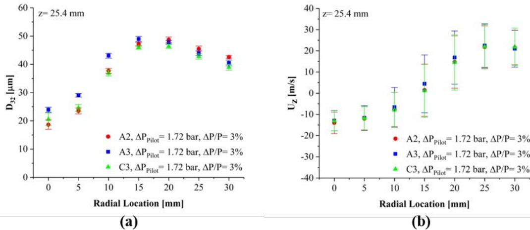
**Figure 9.** Comparisons of  $D_{32}$  and  $U_z$  for A-2, A-3, and C-3 when  $\Delta P/P = 2, 3, 4\%$ ,  $T_{fuel} = 238\text{ K}$ , and  $T_{gas} = 238\text{ K}$  at 25.4 mm measurement plane. Vertical bars on velocity represent RMS.
