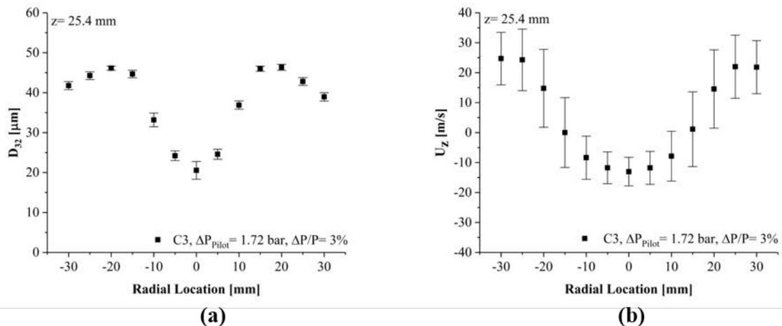
Figure 4.  $D_{32}$  and  $U_z$  distributions for C-3 with  $\Delta P/P = 3\%$ ,  $T_{\text{fuel}} = 238\text{ K}$ ,  $T_{\text{gas}} = 238\text{ K}$  at 25.4 mm measurement plane. Vertical bars on velocity represent RMS.
