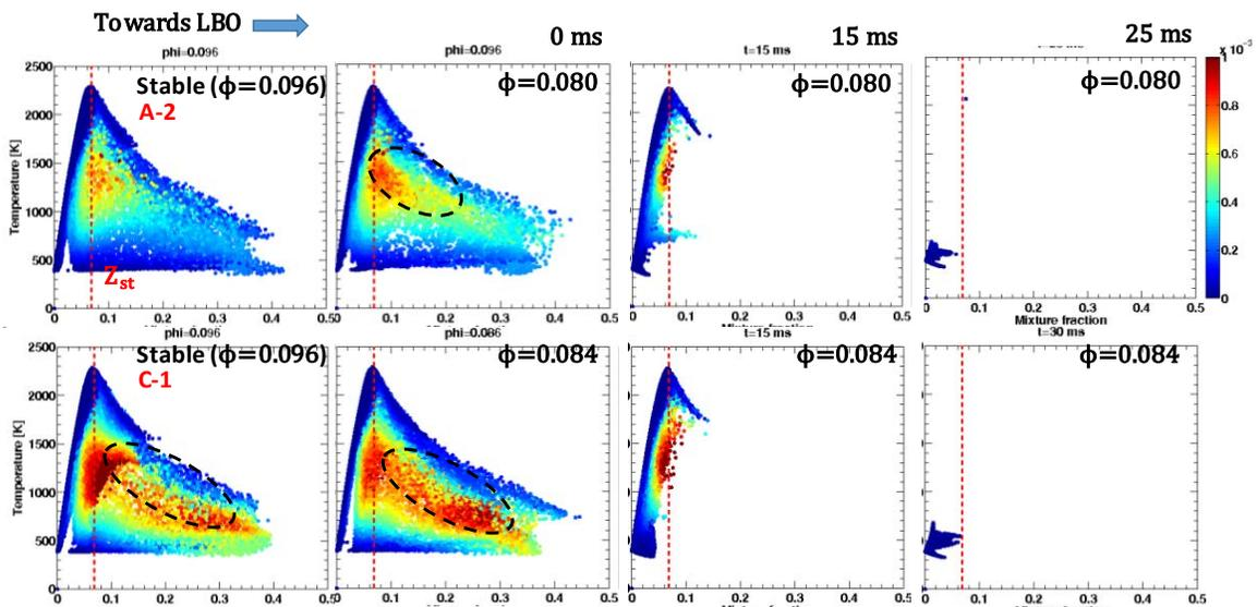
Figure 22. Temperature versus mixture fraction scatterplots for A-2 fuel (top) and C-1 fuel (bottom) sampled from the primary zone. Colored with CH<sub>2</sub>O mass fraction
