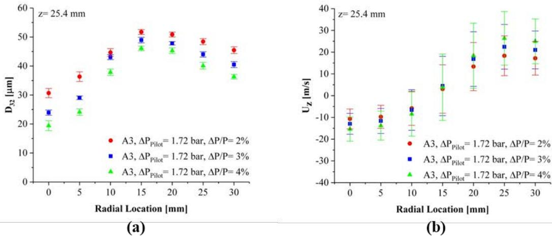
**Figure 7.** Comparisons of  $D_{32}$  and  $U_z$  distributions for A-3 when  $\Delta P/P = 2, 3, 4 \%$ ,  $T_{\text{fuel}} = 238$  K, and  $T_{\text{gas}} = 238$  K at 25.4 mm measurement plane. Vertical bars on velocity represent RMS.
