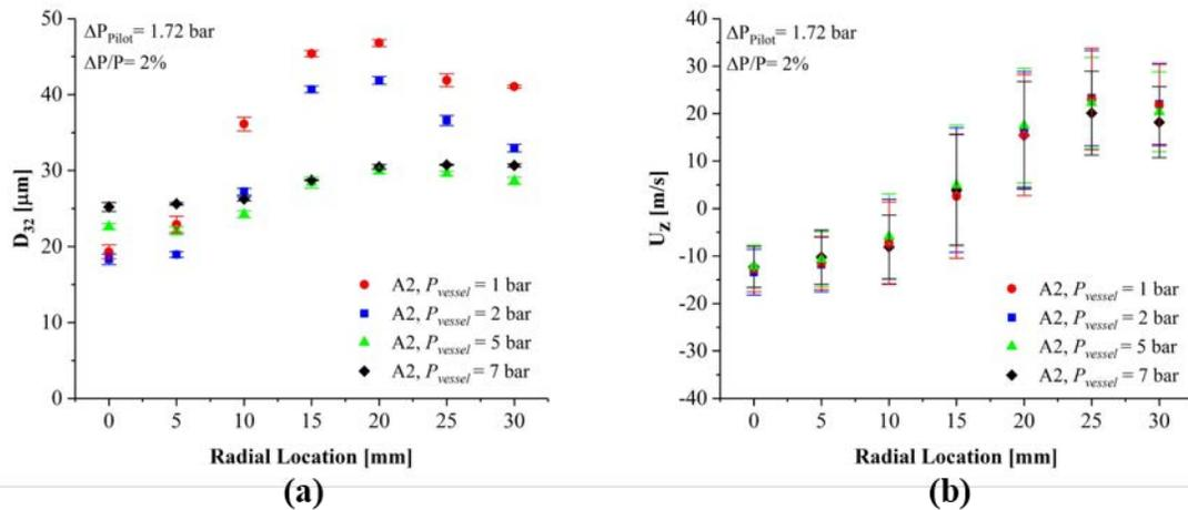
**Figure 10.** Comparisons of  $D_{32}$  and  $U_z$  for A-2 at ambient pressure of 1, 2, 5, and 7 bar when  $\Delta P/P = 2\%$ ,  $T_{fuel} = 278\text{ K}$ , and  $T_{gas} = 259\text{ K}$  at 25.4 mm measurement plane. Vertical bars on velocity represent RMS.
