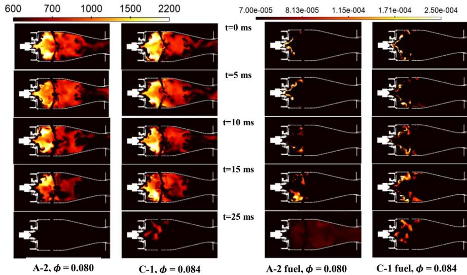
Figure 21. Instantaneous temperature [K] contour plots (left) at the combustor mid-plane and formaldehyde mass fractions (right) for A-2 and C-1 fuel during LBO.
