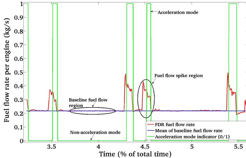
Figure 1. Typical fuel flow rate profile in taxi-out.
