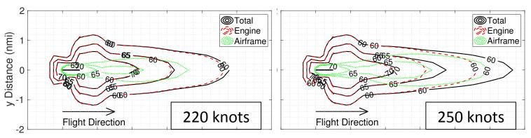
Flaps up airframe noise data from 1970 flight tests (used in the initial MIT analysis of this procedure)
