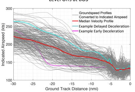
Observed Velocity Variation from Radar Data for B777 4000ft Level Offs at BOS
