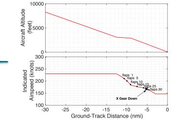
Resulting thrust profile is determined for these profiles from drag data
