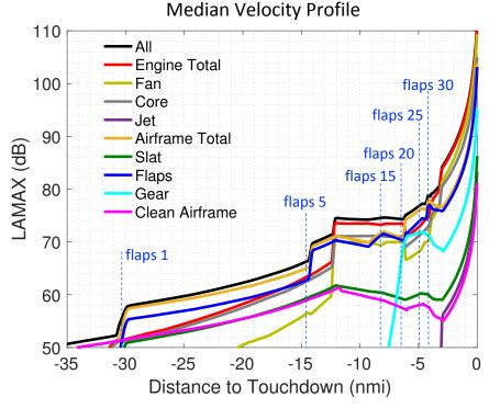
Example Noise Component Breakdown Under the Flight Track for Approach with
