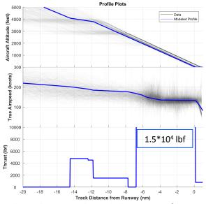
Altitude, speed, and thrust profiles are based on flight profile data from Boston. Slightly adjusted inbound heading
