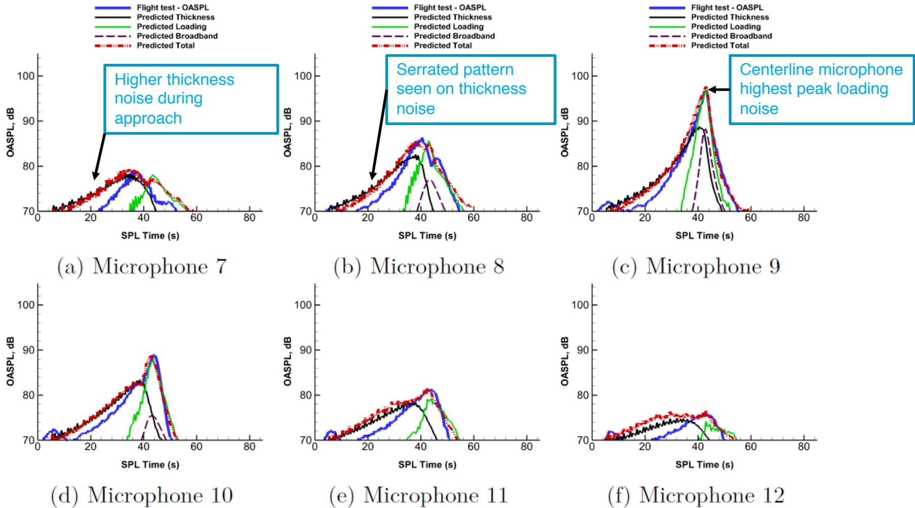
Figure 4.12: Overall sound pressure level along  $x = -304.8$  m for Bell 407 operating at 80 kts level flight.
