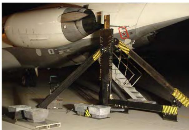
**Figure 1: Probe stand used to sample jet exhaust**
