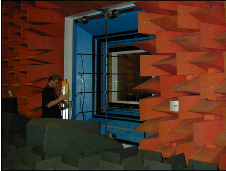
Figure 0.6: Anechoic chamber, view of transmission loss window with Window D installed; computer-controlled intensity probes in foreground.
