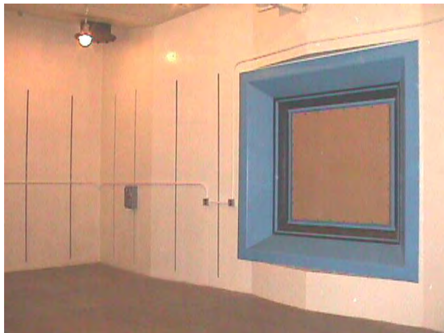
Figure 0.4: Reverberation chamber showing the transmission loss window with a medium density fiberboard panel installed [provided by NASA Langley staff].
