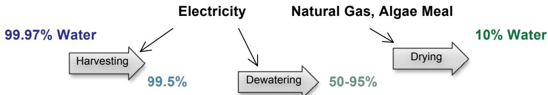
Figure B.10: Flow chart of dewatering and drying of algae
