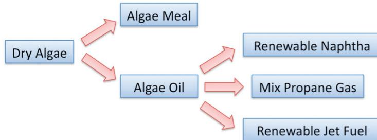
Figure B.8: Co-products that can be created from dried algae. It should be noted that this pathway is the same for palm oil, soybean oil, and many other renewable oil sources. For the allocation methodology used in this analysis, the algae meal is treated as an animal feedstock; however, it could also be used for energy generation.
