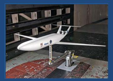
The **"double bubble" D8 Series aircraft design concept** developed by NASA, MIT, Aurora Flight Sciences, and Pratt & Whitney is demonstrating how aircraft configuration changes can provide a **step change in noise and fuel use**
